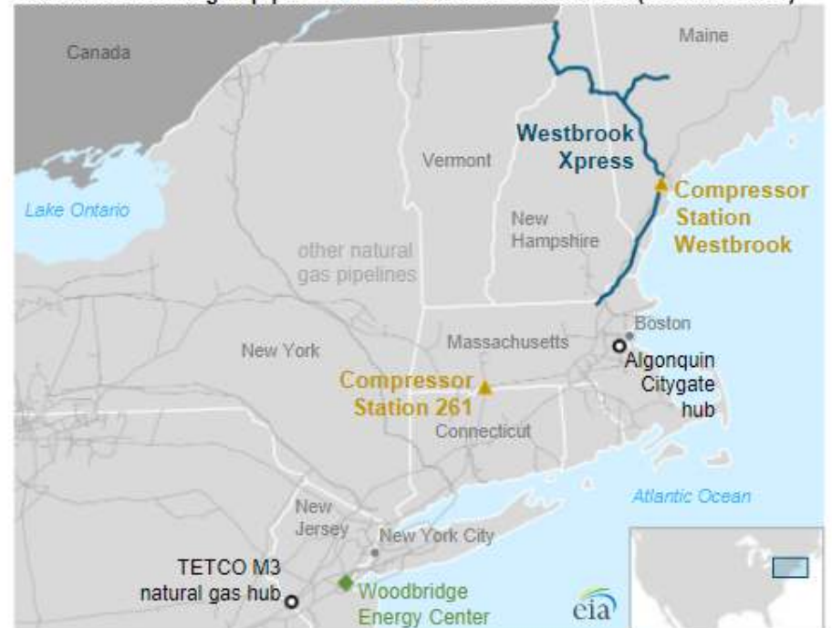
Northeast natural gas pipelines and related infrastructure (October 2021)
